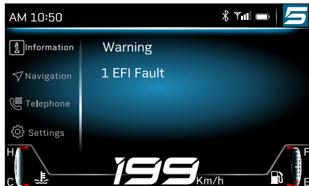
Example with fault.
